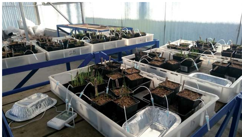
Figure 1: Experimental set up in the green house, plant pots filled with urban wastes as growth substrates
