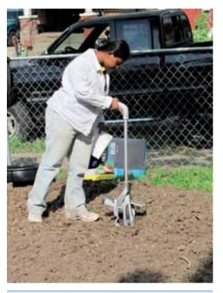
Fig. 5. Conducting preliminary soil tests for total soil trace element concentrations on the Michigan Avenue vacant lot using the field-portable x-ray fluorescence (XRF) spectrophotometer. A handheld GPS was used to record the position of the XRF measurement, and a field notebook was used to record the GPS waypoint and the XRF sampling point number. The data is downloaded from both devices and merged in a spreadsheet.
